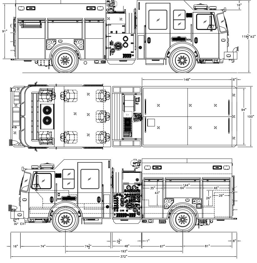
CAB: 100"W KME PREDATOR LFD 16" RR CUMMINS ISX12 500 HP ENG. & ALLISON 4000 EVS TRANS. AXLES: 21,500# FRONT/27,000# REAR
