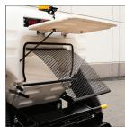
Slide-Out Screen provides easy removal of screen for cleaning.
