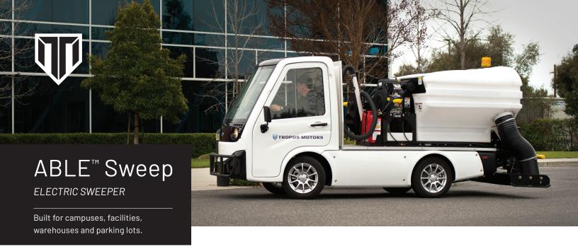
The  $ABLE^{TM}$  Sweep is equipped with the Schwarze<sup>®</sup> SuperVac Aero<sup>TM</sup> and utilizes both the performance and the substantial payload capacity of the ABLE platform to do the work of a full-size sweeper truck.
