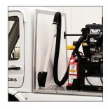
Clean air blower gives operator the ability to remove debris from the curb without additional equipment.
